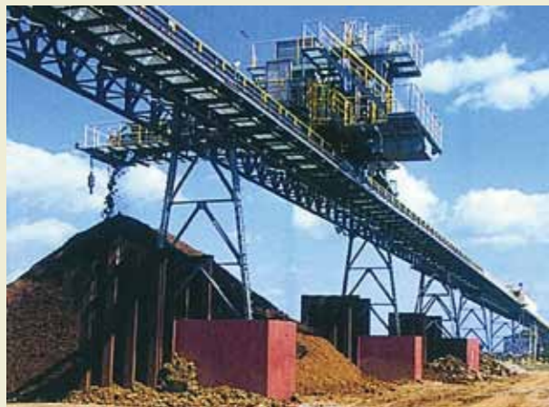
Ore Conveyor: The ore that has been unloaded is transported via 2.4 km long conveyor to the plant.
