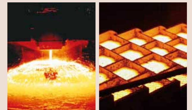
Shot casting: Molten metal is rapidly cooled with water in a water tank and finished into small particles.
