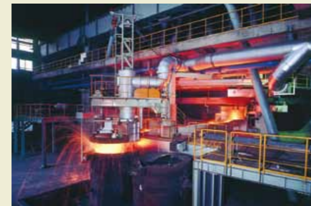
Ferronickel smelting electric furnace: The world's largest class of electric furnace, which smelts ferronickel by melting ore at a temperature of about 1,500 degrees Celsius.
